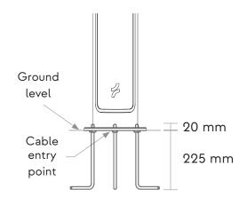
**2.** Place the io7 securely onto the fixings and use a spirit level to ensure the io7 is mounted vertically.
