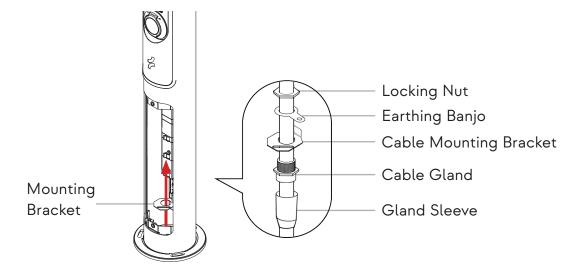
Note: Ensure SWA cable is connected to the Earth block using cable supplied.
