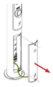
**4.** Install the Steel Wire Armoured (SWA) cable gland to the cable plate, ensuring the Earth tag (banjo loop) is affixed as shown below.
